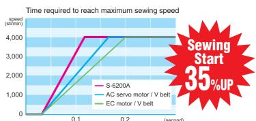
Loss of power transmission has been reduced compared to previous models by equipping the motor behind the machine head and transferring power with the timing belt. Exceptional responsiveness with brother original motor and control box at starting and stopping of sewing will contribute to improving customer's productivity.
