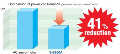
High energy saving with the original motor. The power consumption of S-6200A has been reduced by 41% compared to the V-belt driven system(with an AC servo motor). S-6200A is designed to be efficiently operated with less amount of electricity.
