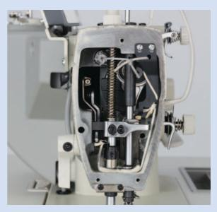
Supplying minimum lubrication to the needle bar and thread take-up area. Oil leakage from the needle bar can be prevented, realizing clean sewing. Also, sewing products will not be stained without V-belt.
