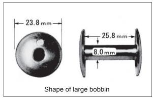
By adoption of large fook, the winding volume of lower thread is increased and due to this feature, the frequency of lower thread replacement is minimized.
